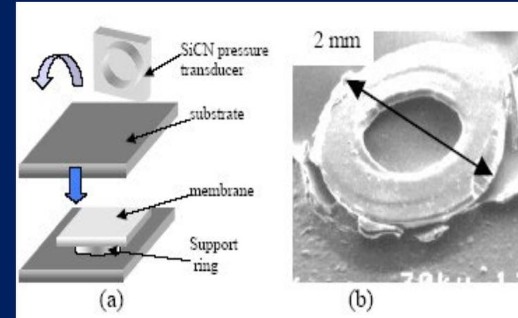
(a) Schematic and (b) SEM pressure sensor
