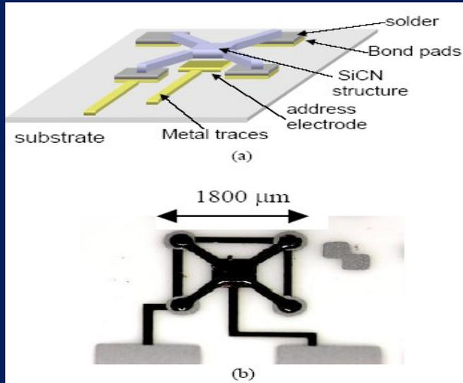
(a) Schematic and (b) fabricated electrostatic actuator
